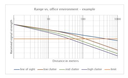
Assumptions: Jabra PRO\*\* 920, US DECT, normal transmit power/long range \*To convert meters to feet multiply by a factor of 3.3
